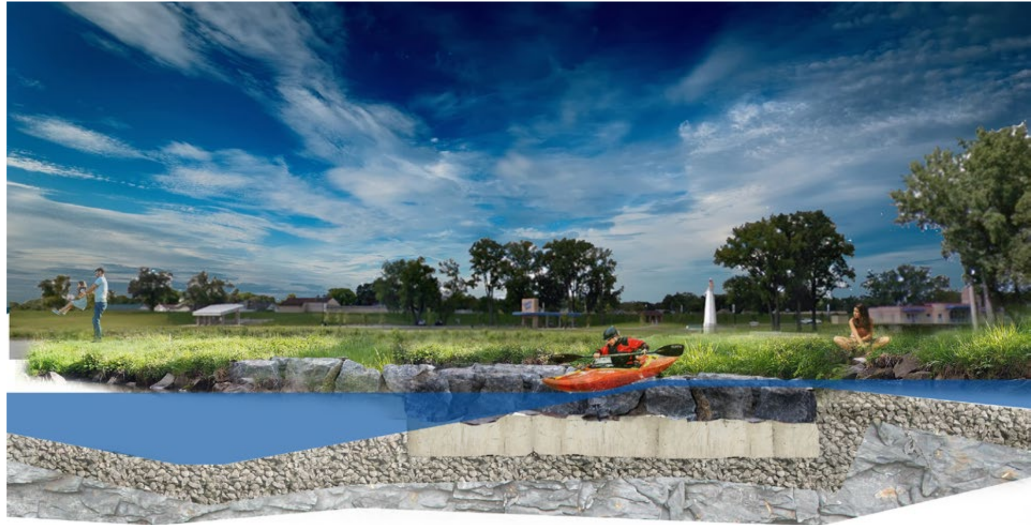
FIGURE 8.4-1 | A cross-sectional view of proposed w-weir at treasure island.
