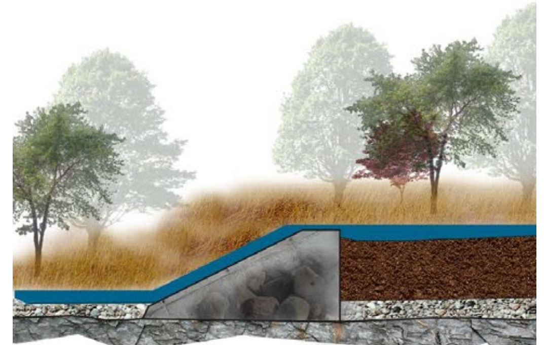
FIGURE 8.1-1 | Diagram of Sediment Dropout Behind Troy Low-Head Dam
