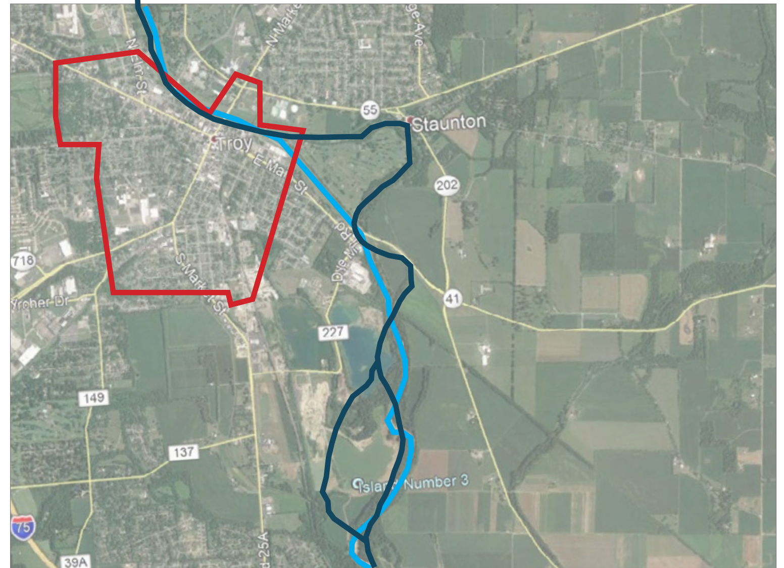
FIGURE 2.6-2 | Troy, Ohio. 2018. — CURRENT ALIGNMENT - GREAT MIAMI RIVER — HISTORICAL ALIGNMENT - GREAT MIAMI RIVER
